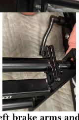
Connect the right and left brake arms and tighten using 13mm wrenches
