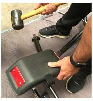
Install the fenders by sliding them over the fender support bracket as shown and lightly tap them with a rubber mallet. You may need to move the hand brake lever tab to fully install the right side fender.
