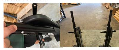
Slide the front yolk assembly into the connection tubes.
