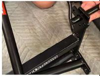
Slide the left side handbrake arm through the left fender support and line up rear connection bracket bottom holes with the two studs on the bottom. Install flat washers nuts and two bolts in the top holes with flat and lock washers. Tighten using a 13mm wrench. Repeat on the right side.
