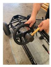
Install spare tire mounting bracket. It simply screws into the frame. Attach the spare tire using the bolt and tighten using a 17mm socket.
