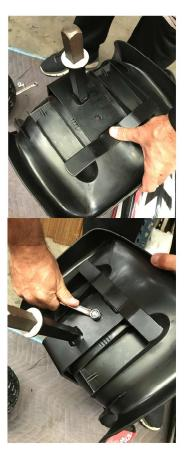
Slide the metal seat frame into the slot on the back of the plastic seat and line up the hole on the seat frame with the hole on the seat.
