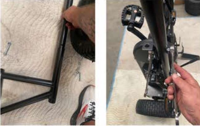
12. Remove hardware from the front yoke. Slide the front yoke over the (2) connector tubes. You may need to pull the rear assemblies together to install the yoke onto both tubes. Be sure that the spare tire mount is facing up.
