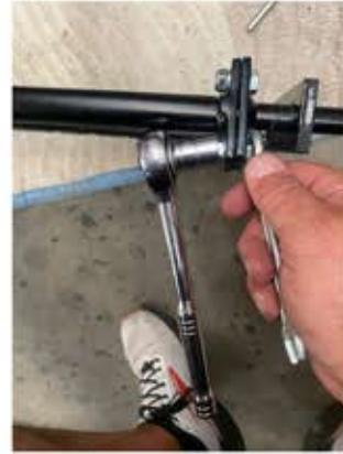
7. Remove the nut and washers from the parking brake cam and install in the hole on the left brace, just below the brake arm. In the resting position, the cam will be on top of the “J” hook. Install so there is a white nylon washer on either side of the bracket, then a metal washer, then the lock nut. **NOTE:Do NOT tighten the lock nut all the way. Tighten until the nut makes contact, then back off 1/2 turn. The brake cam should move up and down freely.**
