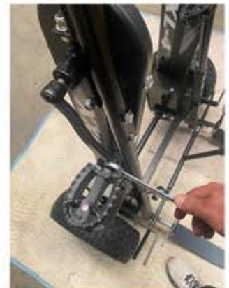
11. Locate (2) front connector tubes and slide into the back frame tube with the larger holes inside. Line up the holes in the tube with the holes in the back frame and install the frame bolt, washer and lock nut. Tighten using 19mm wrenches. Repeat on the other side.
