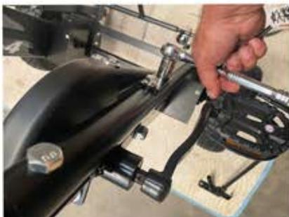
14. Install the end connection that is part of the left side steering shaft into the end of the yoke connector tube. Thread the bolt from the bottom side. Note that there are threads on the top side of the hole. Tighten using a 7mm Allen wrench. Once tight, install the washer and lock nut to the exposed threads and tighten with a 13mm wrench. Repeat procedure on the right side using the single end connection provided.
