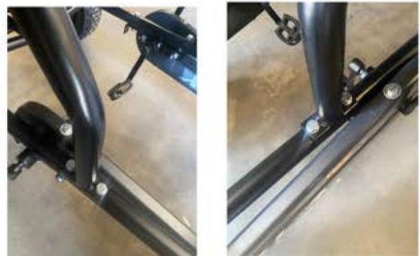
16. Remove the bolt from the end of the passenger grab handle and the bolt from the left steering shaft brace. Slide the grab handle assembly through the right bracing rod and into the end connection. Slide the other end onto left steering shaft brace.
