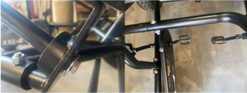
17. Tighten both sides of the rear assembly, (4) bolts and (4) nuts that were not tightened earlier
