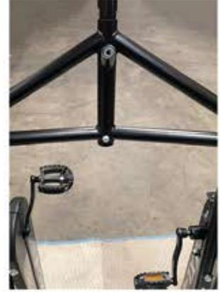
19. Loosen pivot stop bolt on the front assembly and slide the front assembly over the front connection tube. Make Sure the bolt is loose enough for the front assembly to slide all the way onto the connection tube.
