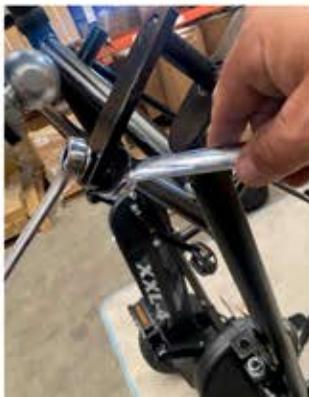
**22.** Remove the bolts from the front axles and slide the (2) coast wheels on the front axles.
