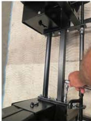
18. Remove the bolt and collar from the front connection tube. Slide the opposite end of the tube through the middle of the front yoke and line up the holes.
