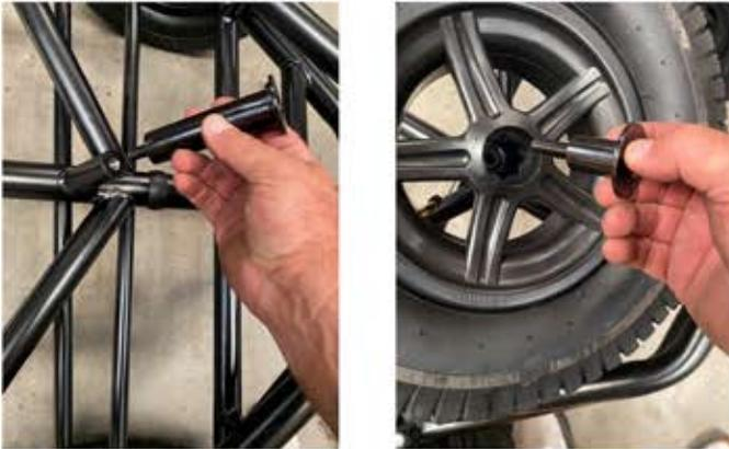
The spare wheel can be used for either the drive or coast wheel as a spare. But the bearings or bushing from the wheel being replaced must be installed into the spare wheel before use.
