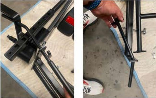
5. Remove the (2) nuts and washers and (2) bolts and washers from the rear frame on both sides. Next, insert the hand brake through the support bracket of the rear assembly.. Install the nuts and bolts connecting the rear frame connector to the right and left rear frame. **DO NOT TIGHTEN**
