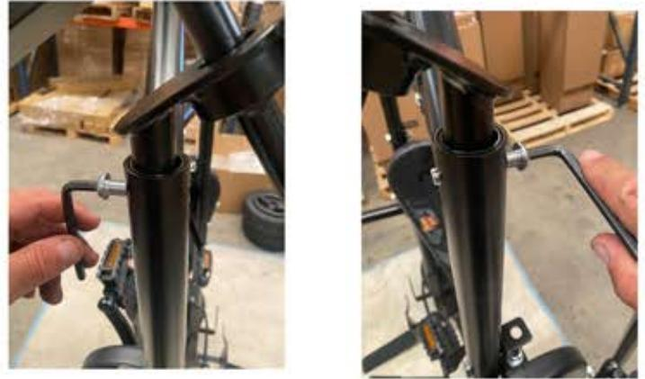
15. Line up the holes for the left bracing rod that is part of the steering shaft assembly, re-install the (2) bolts and washers and tighten using a 17mm wrench. Next, install the right bracing rod, re-install the hardware and tighten.
