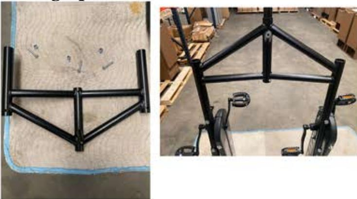
13. Remove steering bracing arm bolts from each side.
