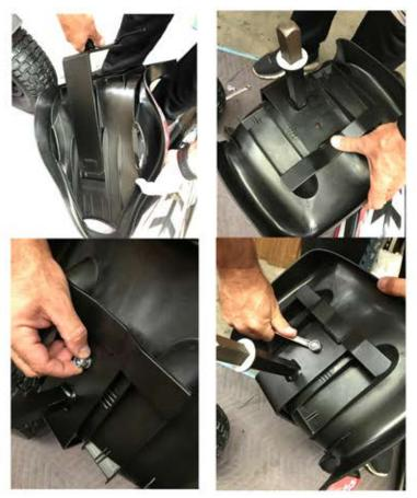
Slide the metal seat frame into the slot on the back of the plastic seat and line up the hole on the seat frame with the hole on the seat.
