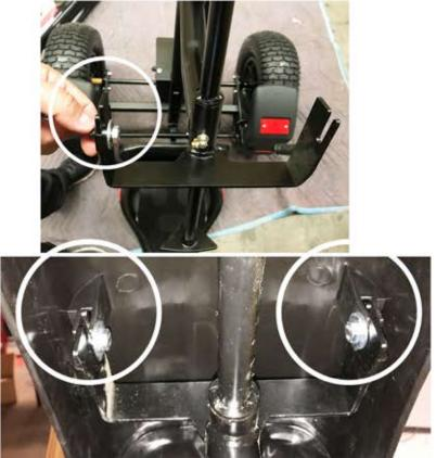
17. After the bolts are tight on the top of the spoiler mount, tighten the screw at the bottom of the spoiler using a Phillips screwdriver.
