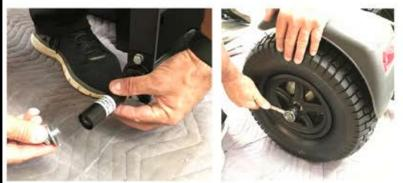
Using a 17mm socket, remove the bolt and washer from the coast side of the rear axle and remove ONLY the metal spacer from the axle (not the plastic spacer) Slide the coast wheel on the axle with the air fill valve facing INWARD.
